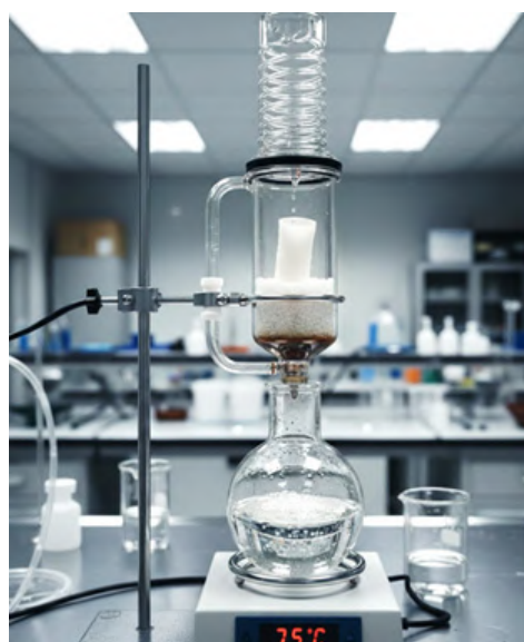
Figure 4: Soxhlet extraction of vascular graft
